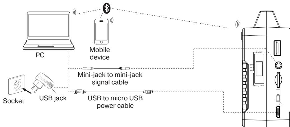
Fig. 2. Connection diagram
