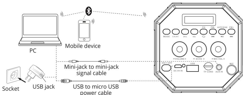
Fig. 2. Connection diagram
