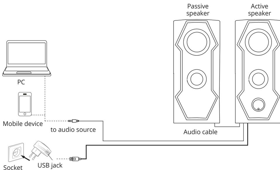
Fig. 2. Connection diagram
